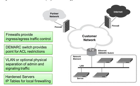
A DSR node consists of a suite of servers and related Ethernet switches that create a cluster of servers, operating as a single Network Element. It is assumed that the service provider
